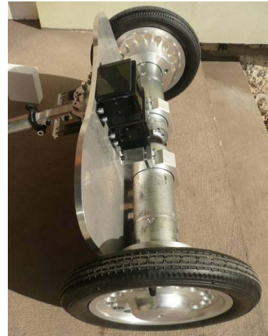
Figure 5. Detailed view of DC motors and wheel mounting
