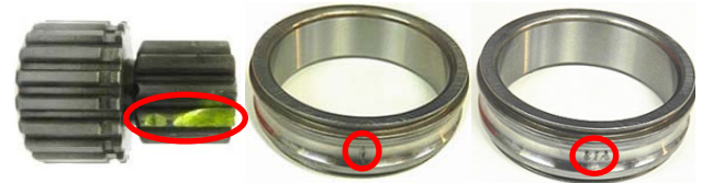
Figure 2. Tooth defects simulated on the sun gear and two kinds of inner race defect on deep groove ball bearing
